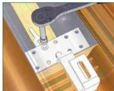
Mounting with aluminum underlay shims
